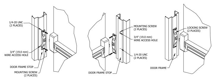
NOTE: Wire access hole locations are relative to the exit device orientation.
